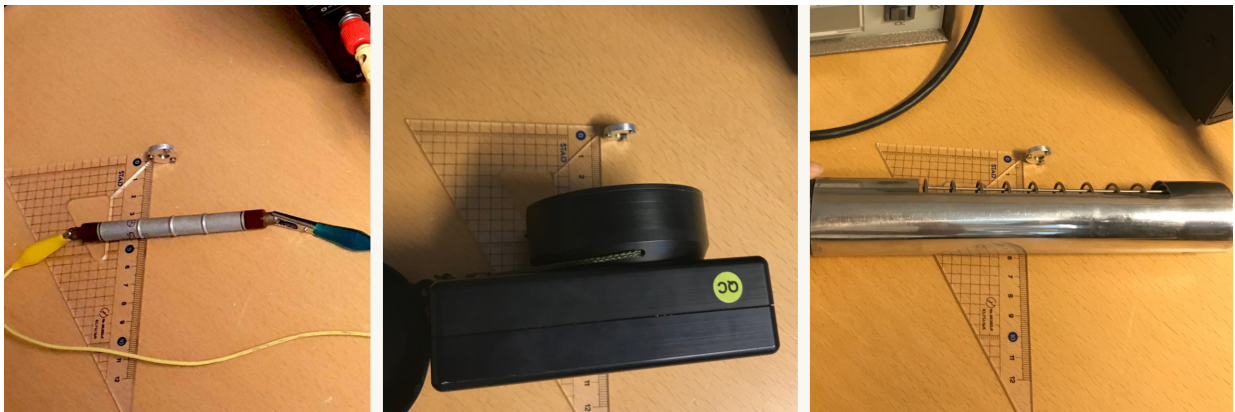
Figure 9: The setup for the radiation measurement test using our Geiger-Müller counter (left), RAM GENE-1 (middle) and Mini-Monitor G M Meter (right)
