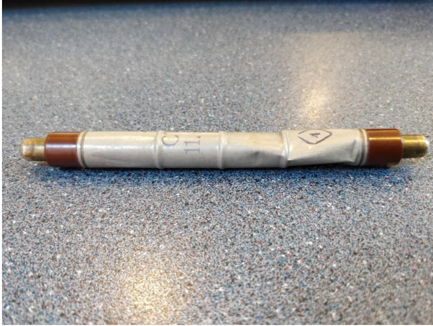
Figure 14: The GM tube after the first cooling test.
